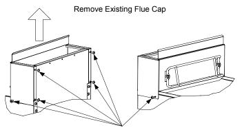
Remove the six screws (four in the back and one in each side corner) and lift the flue cap from the fryer.
