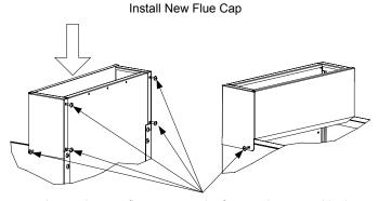
Lower the new flue cap onto the fryer and secure with six screws (four in the back and one in each side corner).
